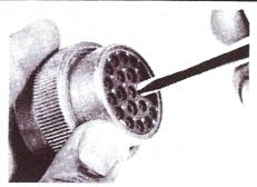
until it engages contact and resistance is felt. NOTE: Do not twist or insert tool at an angle.
