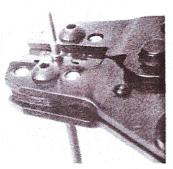
3. Close ratchet until terminal is secure and will not fall out. Place the stripped end of the wire in the crimp barrel and fully depress the tool handles. Release, and remove. If tool does not release, press further on handle.
