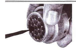
1. With rear insert toward you, snap appropriate 2. Slide tool along wire into the insert cavity size extractor tool over the wire of contact to be removed.
