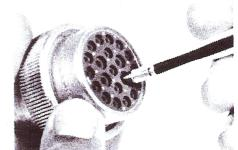
3. Pull contact-wire assembly out of connector.
