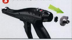
Insert small end of the calibration tool into knob and align with holes in tension adjustment nut.
