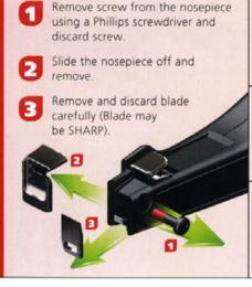
Install new blade by aligning the chamfered (beveled) corner with the housing.
